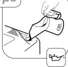
Clean around the oil filler cap before removing. With the mower on a level surface, unscrew and remove the oil filler - dipstick. Wipe oil from it with a clean cloth. Screw the oil filler - dipstick back in place, then unscrew and remove it to check the oil level.
